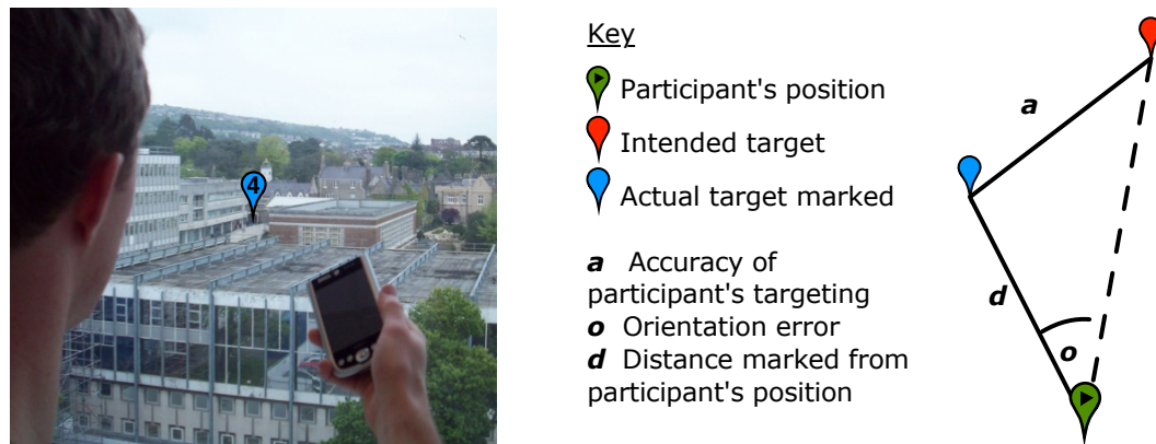
FIGURE 3.4: Left: marking a target from the position participants stood at in the lab. Right: accuracy measurements recorded for each point marked by participants during the study.
