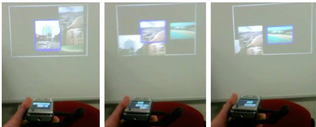
FIGURE 4.2: The prototype in use, showing a user selecting content from a cluster of images by pointing the device itself. Sensor data is used to correct for device movements and image skew to allow selection of individual items by moving the device, rather than a pointer. The current selection is highlighted by the system in each image.
