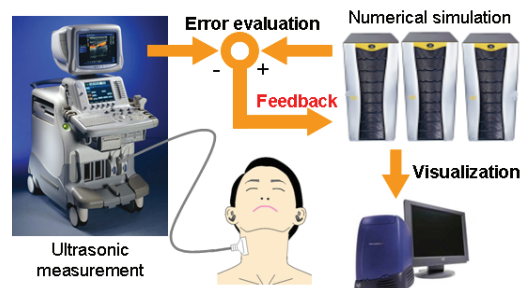
Fig. 1. Schematic diagram of UMI simulation system.
