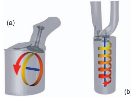
Fig. 13. Idealized in-cylinder flow through a gas engine (a) and a diesel engine (b). Figs. 14 and 2 show our visualization of CFD data simulating such flows.
