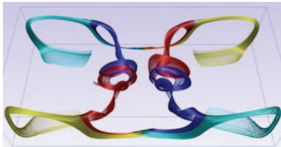
Fig. 5. Our similarity measures and clustering algorithm segment the streamlines on this rake into distinct, intuitive clusters. Two rakes were used to generate two sets of streamlines on a simulation of Bénard convection in this image. Color indicates cluster membership. Note colors are re-used for each rake (i.e. the two red clusters are distinct clusters).
